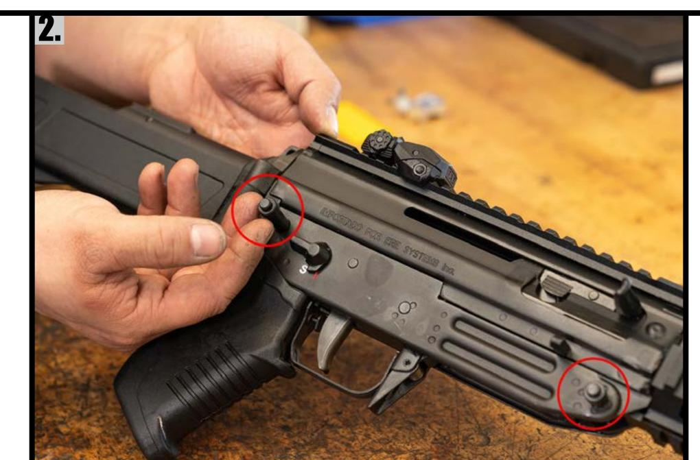
(2) REMOVE THE TWO RETENTION PUSH-PINS FROM LOWER RECIEVER
